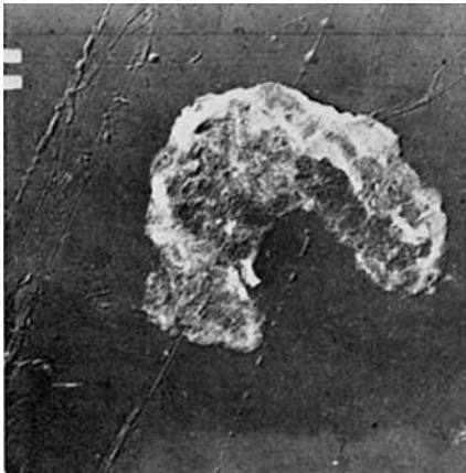
Fig. 10. Electron micrographs taken after 30 min. immersion in Cuene of ultrathin sections of cotton fiber treated with DMEU in the presence of 0.03 M \text{MgCl}_2 and 0.03 M \text{Zn}(\text{NO}_3)_2 at 45, 55, and 65°C. (10A) \text{MgCl}_2 at reaction time of 1500 minutes; (10B) \text{Zn}(\text{NO}_3)_2 at reaction time of 200 min. Magnification: 3240 \times .
